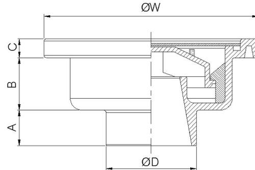
Light duty residential applications this drain is furnished with ABS body and stainless steel grate. And odor protection by water trap. Fit for pipe inside  $\text{Ø}1.5''$  to  $\text{Ø}3''$
